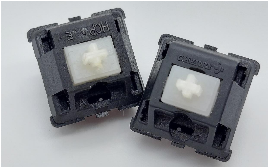
Figure 21: Cherry Hirose Clear and HCP Hirose Clear switches. (Contrast increased to show nameplate design.)
