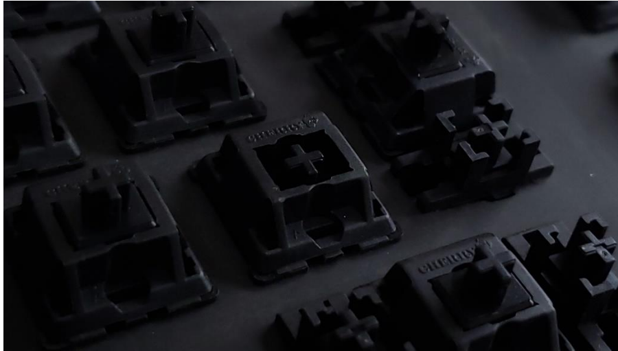
Figure 12: Dummy Stabilizer MX Black switch from a BAE key. Photo courtesy of vintage collector mcmaxmcmc.
