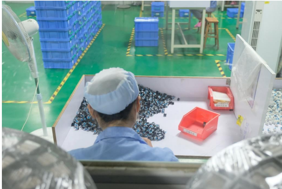
Figure 8: Photo from inside Gateron manufacturing facility showing hand inspection of switches by employees.
