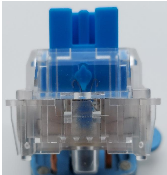
Figure 25: Snap spring mechanism from the front side of a large GTMX display switch.
