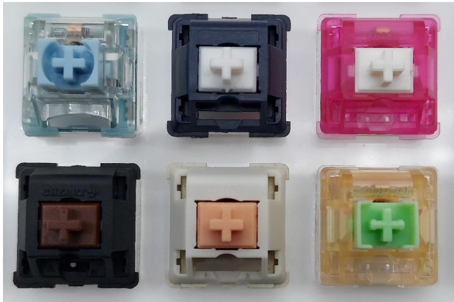
Figure 18: Switches for comparison. (L-R, Top-Bot: TTC Blueish White, Naevy V1.5, C3 Equalz Dragonfruit, Cherry MX Brown, Massdrop x Invyr Holy Panda, Gateron Kangaroo Ink)
