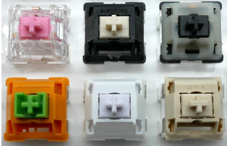
Figure 14: Switches for comparison. (L-R, Top-Bot: Tecsee Honey Peach, Sarokeys BCP, Cherry MX2A RGB Black, Huano Pineapple, Wuque Studio Morandi, and Novelkeys Cream)
