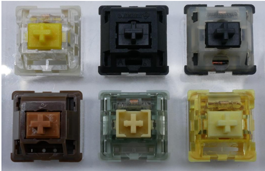
Figure 31: Switches for comparison 2: Electric Boogaloo (L-R, Top-Bot: KTT Custard, Cherry MX Black, Cherry Nixdorf Black, Chocolate Toffee Linear, Huano Spirit Wind, Akko V3 Cream Yellow)
