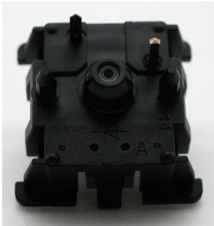
Figure 10: Cherry MX Purple bottom housing external design showing five pin/PCB mount style and two part mold markings in lower right-hand corner.
