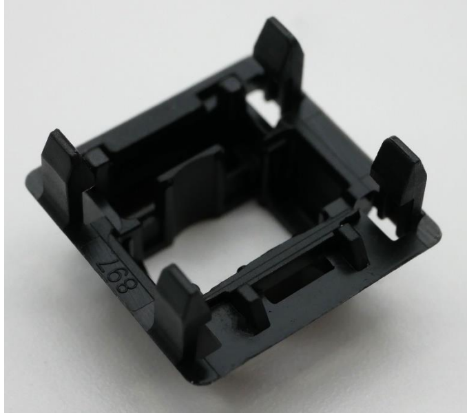
Figure 9: Cherry MX Purple top housing internals showing similarities to other MX2A platform switch housings as well as its triple digit mold marking on left hand edge.
