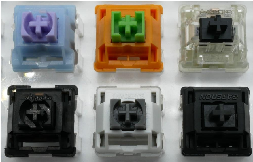
Figure 9: Switches for comparison. (L-R, Top-Bot: Moyu Studio x XCJZ Snow Grape, Huano Pineapple, Cherry MX2A RGB Black, Obsidian Pro, Invokeys Black Sesame, and Gateron Oil King)
