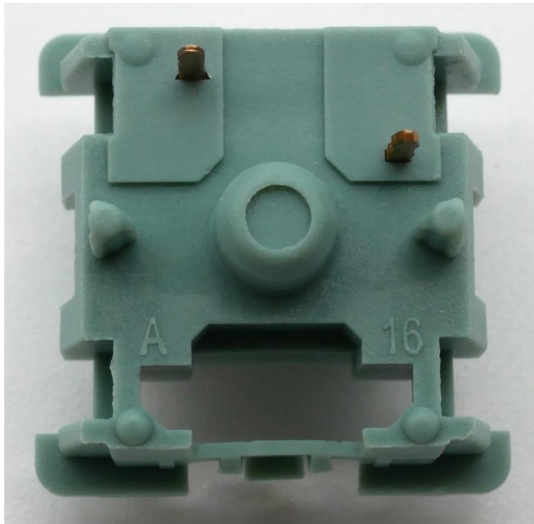
Figure 7: Feker Emerald Cabbage bottom housing external design showing pair of mold markings in lower corners and PCB mounting pins.
