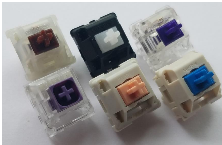
Figure 5: Switches for comparison. (L-R, Top-Bot: Gateron RGB Brown, Cherry MX Clear, Zealio V1 (62g), Box Crystal Royal, Massdrop x Invyr Holy Panda, and Novelkeys Blueberry.)
