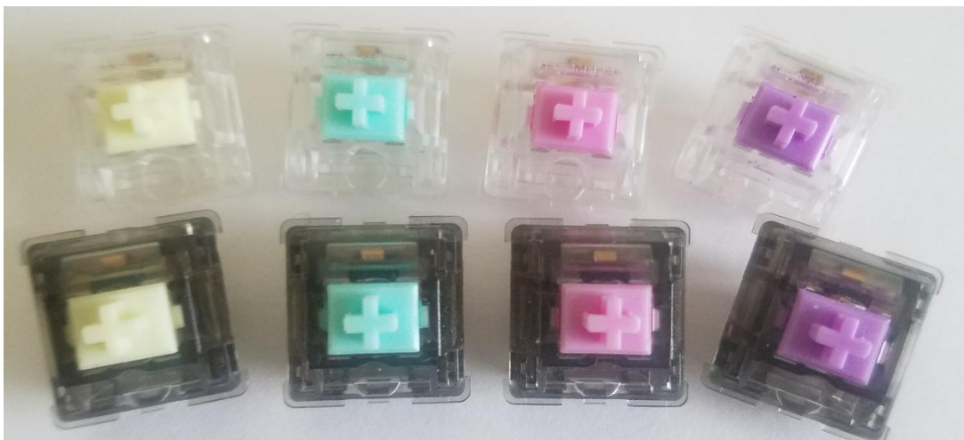
Figure 1: Picture of real Geekmakers (back) and the fake Geekmakers (front) acquired directly from a Durock sales rep.
