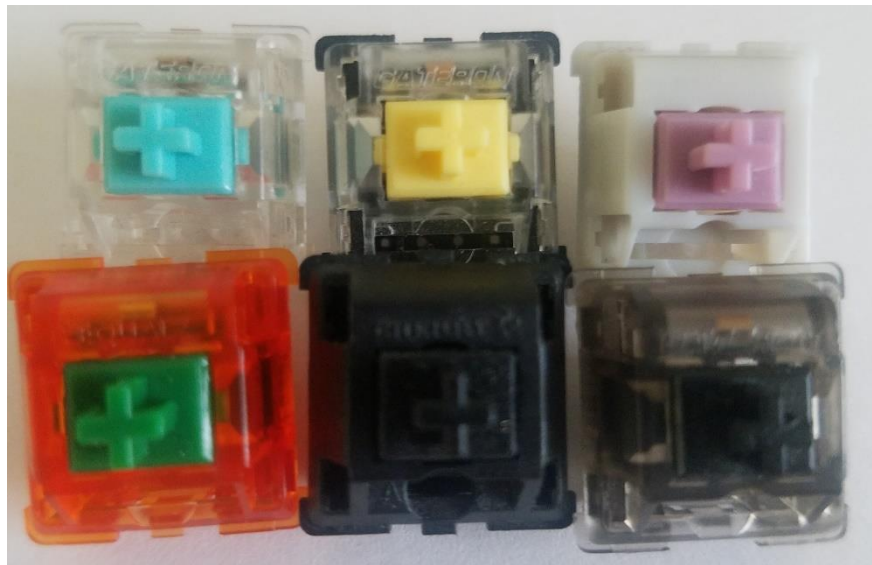
Figure 4: Switches being compared to Geekmakers. (Back, L-R: Tealios V2, Gateron SMD Yellow, Mauves. Front, L-R: C 3 Equalz Tangerine V2, Cherry MX Vintage Black, Gateron Ink V1)
