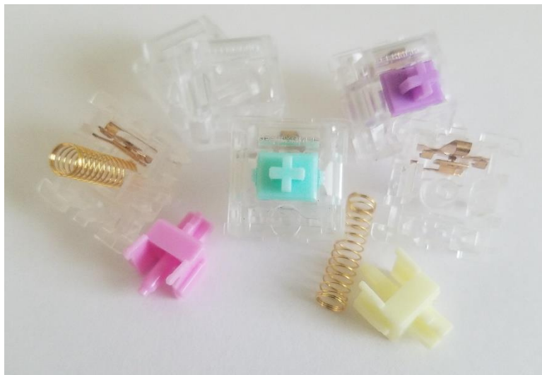
Figure 3: Picture of the springs, stems and housings of the Geekmaker switches conveniently placed here because it was too close to the last picture if placed right after the 'Appearance' section.
