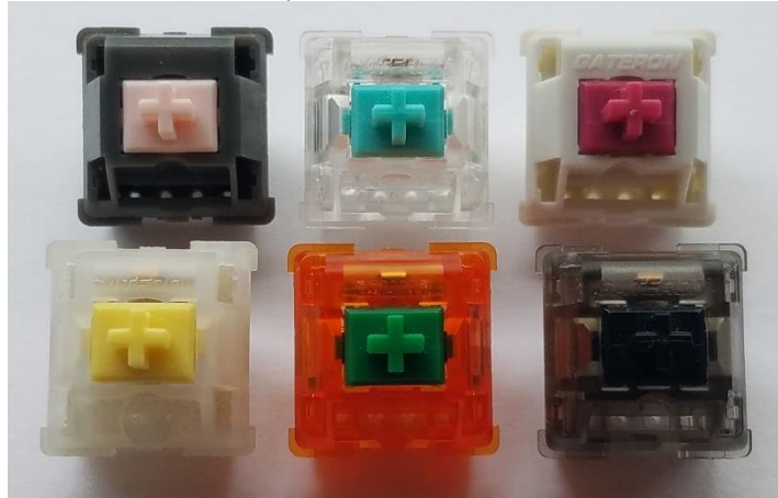
Figure 7: (Top-Bot, L-R) Switches used for comparison: Alpaca, Tealio V2, Gateron Merlot, Gateron Milky Yellow, C 3 Tangerine V2, and Gateron Ink V1.
