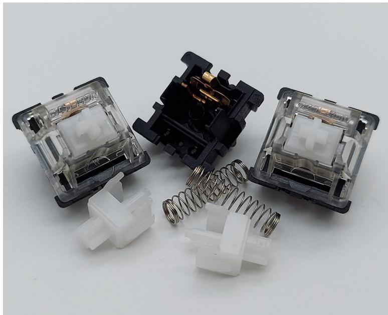
Figure 5: Winkeyless.KR Zeal Clear switches and components.
