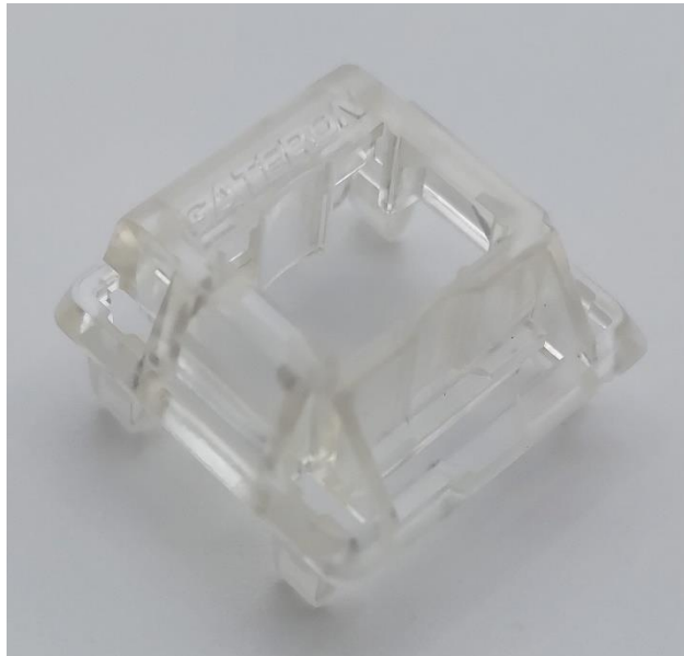
Figure 8: Winkeyless.KR Zeal Clear top housing external side showing traditional Gateron nameplate and wide channel LED slot.
