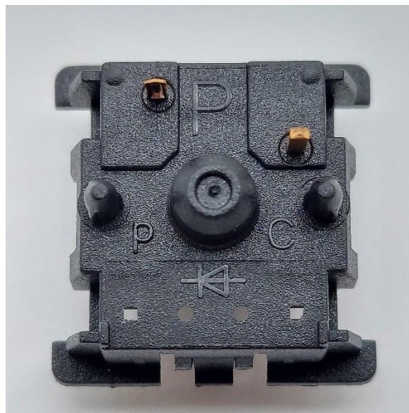
Figure 6: Winkeyless.KR Zeal Clear bottom housing external shot showing various mold markings and LED slot design.
