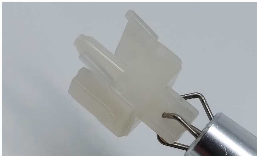
Figure 3: Front side of the UHMWPE Hippo stem showing front plate mold circles.
