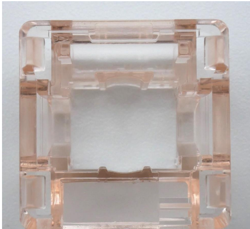
Figure 7: Gateron Melodic top housing internal design showing mold markings in upper left- and right- hand corners as well as underside of asymmetrical LED bubble with outcropping for compacting the click leaf.
