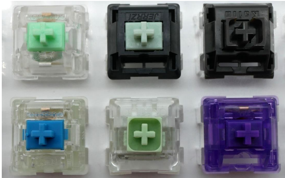
Figure 14: Switches for comparison. (L-R, Top-Bot: Zeal 3-in-1 Clickiez (40g), XCJZ Jerrzi Lotus Stem, Novelkeys Cream Clickie, Cherry MX2A RGB Blue, Kailh Box Jade, and TKC Blackberry)
