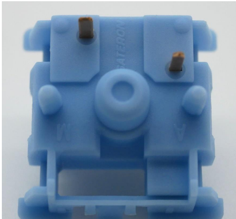
Figure 11: Gateron Melodic bottom housing external design showing 5-pin/PCB mounting posts, anticounterfeit mold marking between the metal PCB pins, and LED slot asymmetry from the click leaf mechanism.
