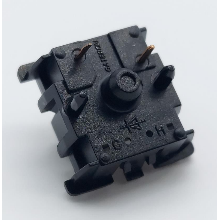
Figure 9: Gateron Oil King bottom housing external design showing mold markings and 'Gateron' anticounterfeit stamp.
