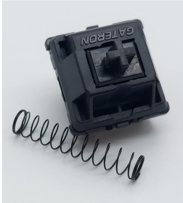
Figure 6: Gateron Oil King switch with stock, black 22 mm. long spring.
