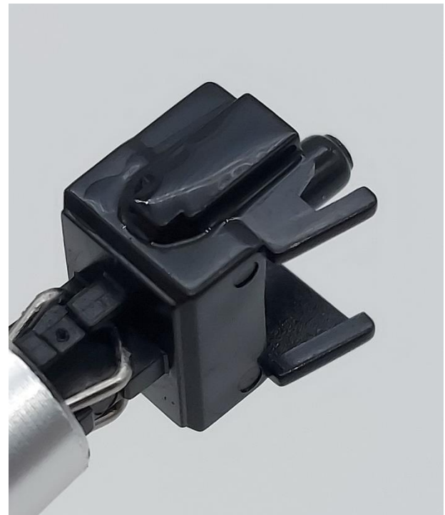
Figure 7: Gateron Oil King stock lubrication demonstrated on stem.
