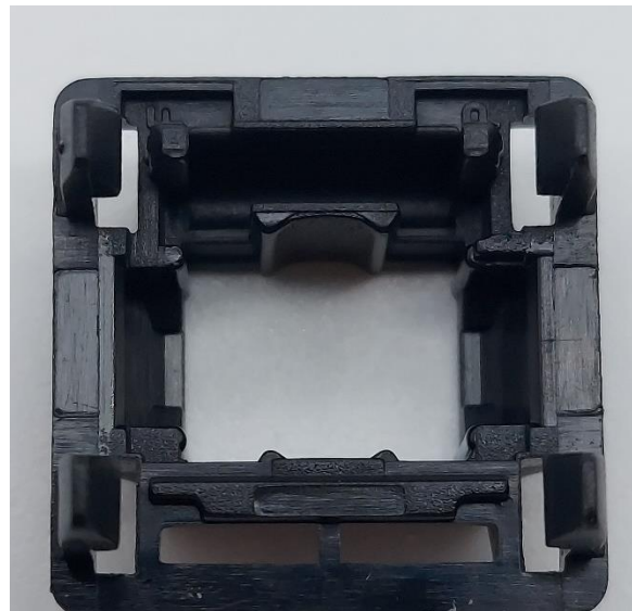
Figure 9: Gateron Oil King top housing internal design showing two single-letter mold markings in the upper corners.
