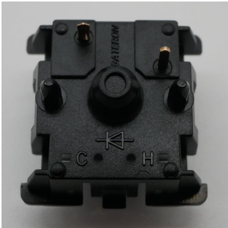
Figure 8: Gateron UHMknown bottom housing external design showing 'GATERON' anticounterfeit stamp and pair of capital letter mold markings between LED and diode pin outs.
