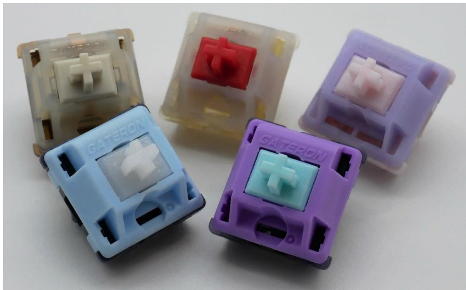
Figure 5: Custom designed Gateron switches with ink thermoplastic material including Root Beer Float, Cream Soda, Malvix Studio Irene, Mizu Mink, and Blue Bubblegum.
