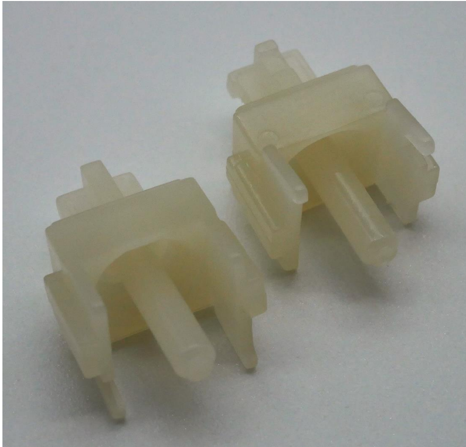
Figure 7: Gateron UHMknown stem front and back showing front plate mold ejector circles, non-tapered slider rails, and short, untapered center pole.
