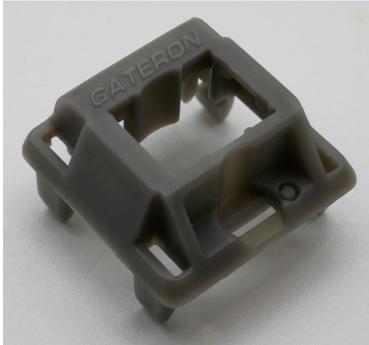
Figure 7: Gateron UHMknown top housing external design showing normal facing nameplate and extremely restricted through-switch LED slot.
