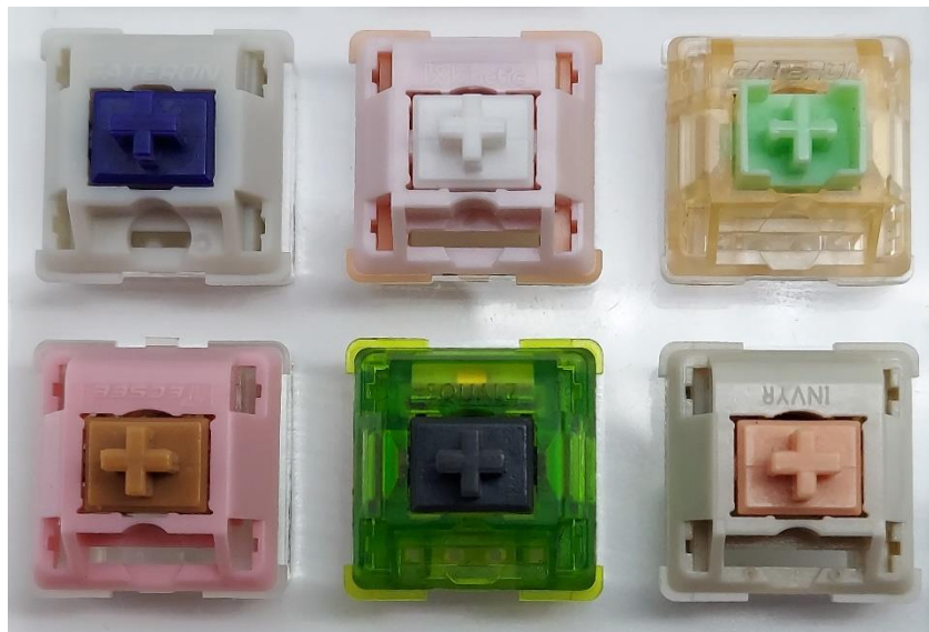
Figure 19: Switches for comparison. (L-R, Top-Bot: Zealio V1 Redux (67g), Salmon, Gateron Kangaroo Ink, Neapolitan Ice Cream, Kiwi, Massdrop x Invyr Holy Panda)
