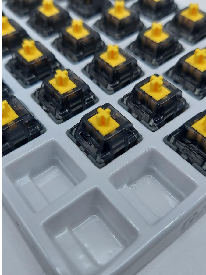
Figure 18: Close up of the tiered wells in the plastic switch holder tray provided in Holy Panda X packaging.
