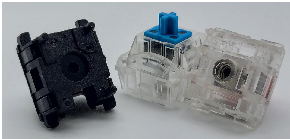
Figure 6: Gateron KS-5 'Hammer over Membrane' underside design next to TTC MT switches with same mechanism.
