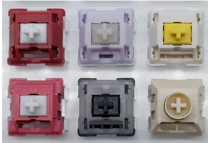
Figure 16: Switches for comparison. (L-R, Top-Bot: Raed, Gateron Hippo, Novelkeys Silk Yellow V2, KTT Grapefruit, Opblack, Novelkeys Box Cream)
