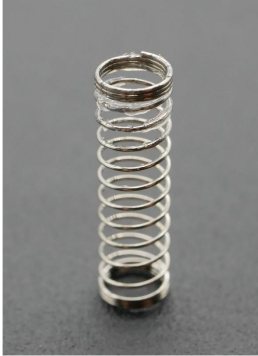
Figure 18: Upside-down Invokeys Blueberry Chiffon spring image showing factory lubrication around bottom side of the spring.
