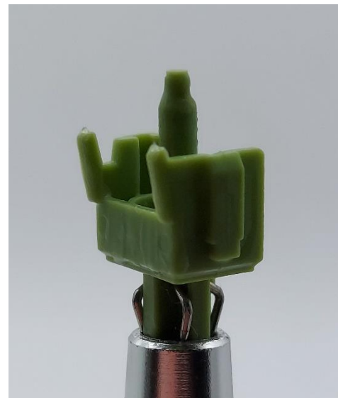
Figure 13: Matcha Latte stems showing tapered slider rail, tapered central pole, and factory lubrication.
