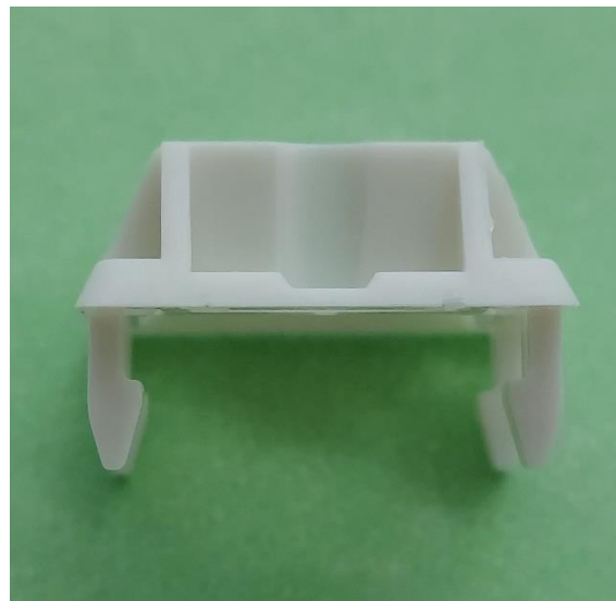
Figure 10: Matcha Latte top housing edge 'chipping' defect.
