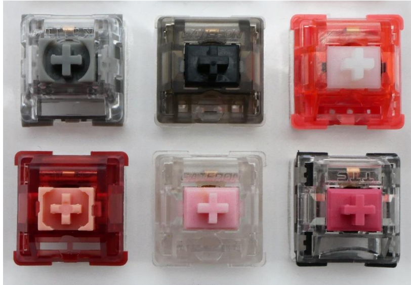
Figure 17: Switches for comparison. (L-R, Top-Bot: Kailh Midnight Pro Grey, Gateron Silent Ink V2, Silent Coral, Haimu Heartbeat, Sakurio, TTC Silent Red V2)
