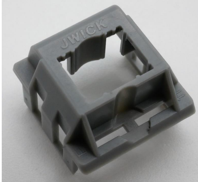
Figure 7: JWICK Semi Silent top housing exterior design showing JWICK nameplate, odd mold marking locations, and bifurcated LED slot.
