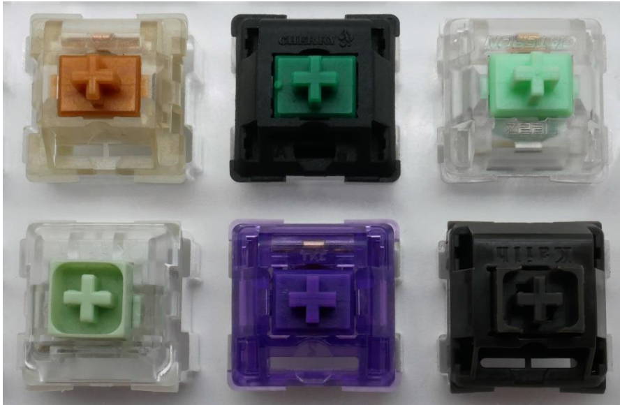
Figure 21: Switches for comparison. (L-R, Top-Bot: KTT Gold, Cherry MX Green, Zeal 3-in-1 Clickiez (40g), Kailh Box Jade, TKC Blackberry, and Novelkeys Cream Clickie)
