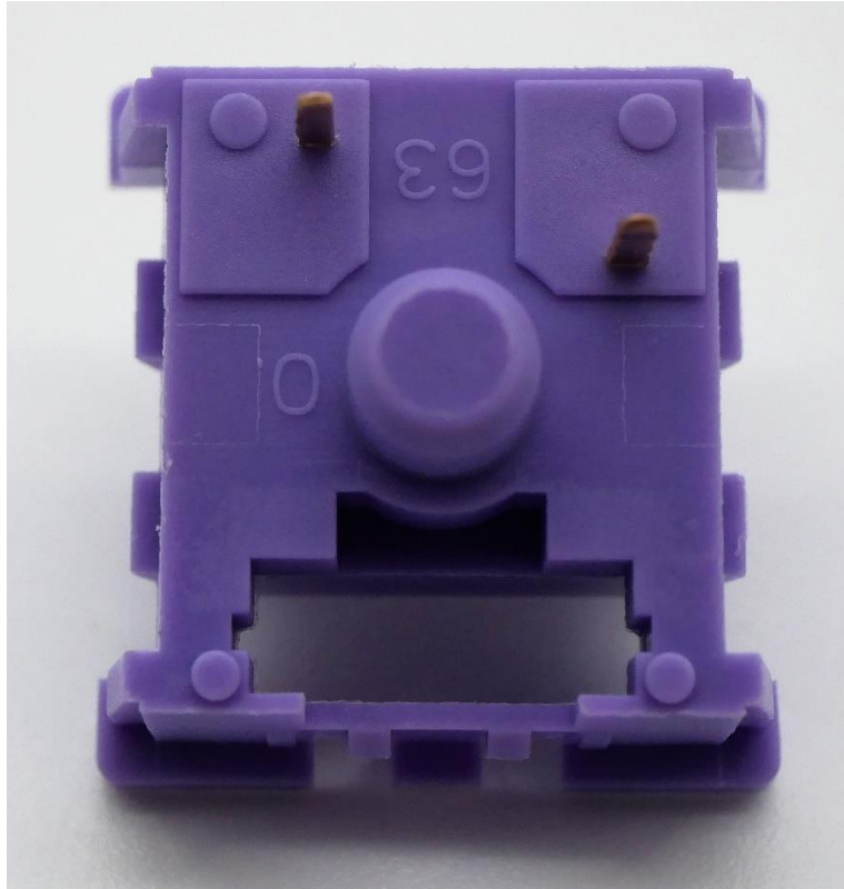
Figure 15: KTT Purple Sauce bottom housing exterior design showing three pin construction and two locations of KTT-specific mold markings.
