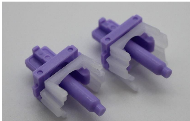
Figure 12: Front and back side view of KTT Purple Sauce stem showing articulation of click jacket mechanism and mold ejector circles.
