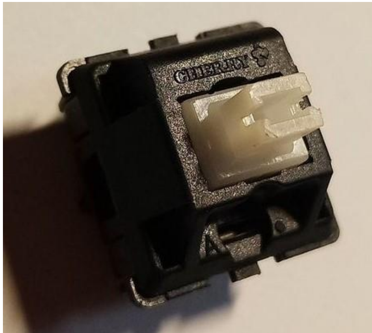
Figure 5: Image of the questionably authentic Cherry MX-made Alps mount switch.
