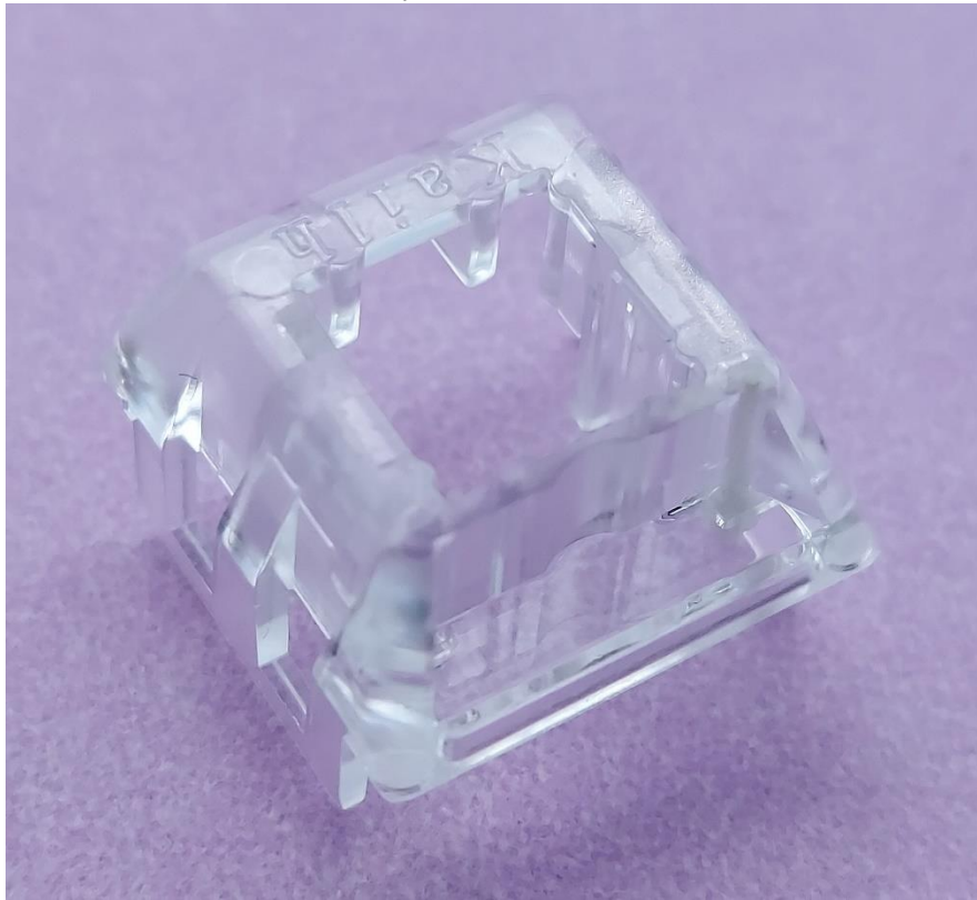
Figure 6: Kailh Box Mute Jade top housing externals showing flipped nameplate, thick covered LED slot, and muting bar mechanism in the front right-hand corner.
