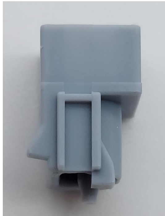
Figure 8: Kailh Box Mute Jade stem showing externally facing clickbar stem leg (left) and internally facing activation lever stem leg (right).
