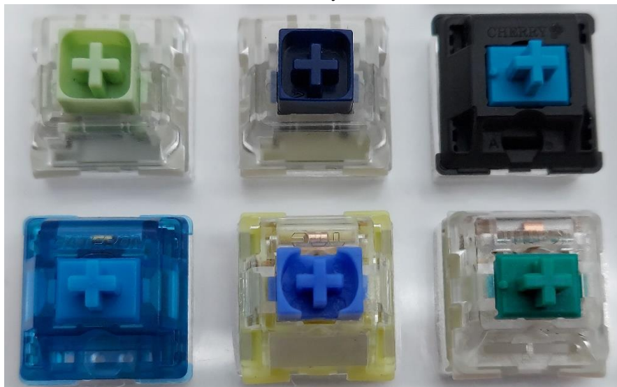
Figure 13: Switches for comparison. (L-R, Top-Bot: Kailh Box Jade, Kailh Box Navy, Cherry MX Blue, Gateron Blue Ink V2, TTC Brother, Kailh Pro Light Green)
