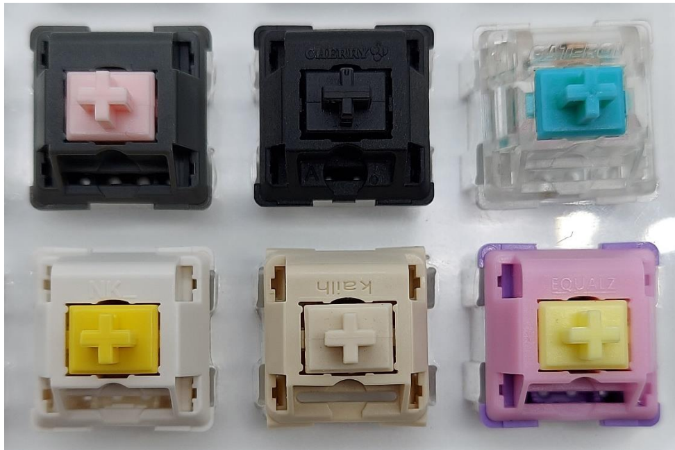
Figure 12: Switches for comparison. (L-R, Top-Bot: Alpaca V2, Cherry MX Black, Tealio V2, Novelkeys Silk Yellow V2, Novelkeys Cream, C3 Macho)
