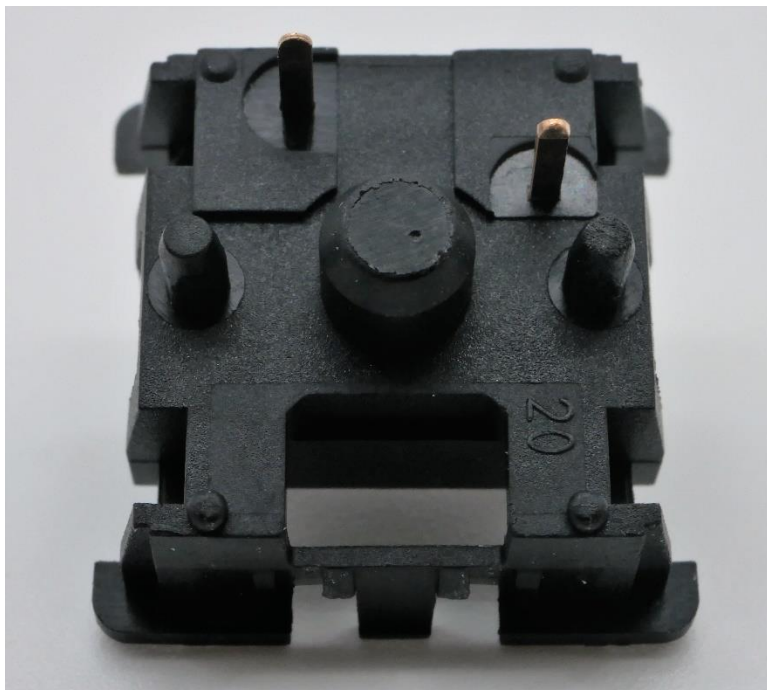
Figure 7: MODE Tomorrow bottom housing externals showing off square-like LED slot bottom, double number mold marking, and PCB mounting pins.
