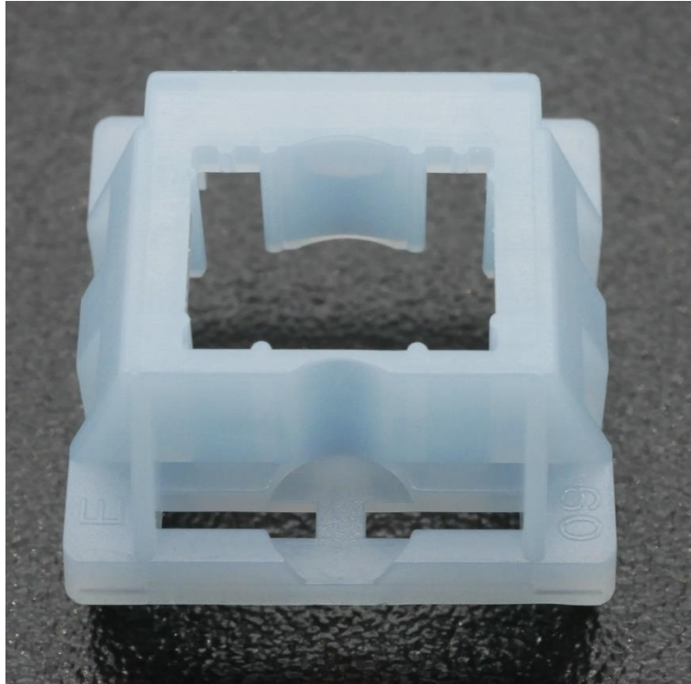
Figure 7: Moyu Studio x XCJZ Snow Grape switch top housing external design showing bifurcated LED slot design and left- and right-hand mold markings surrounding it.
