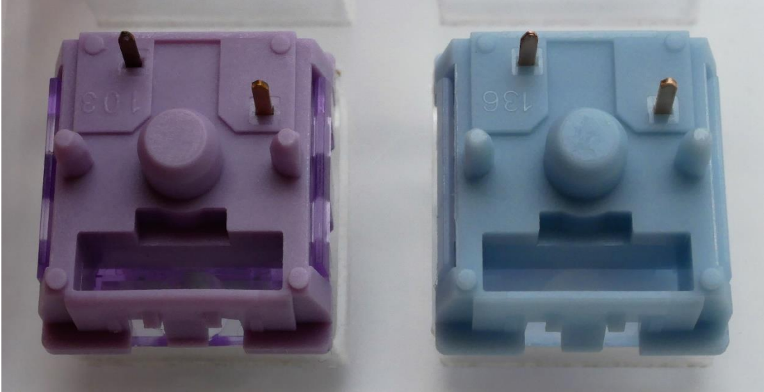
Figure 8: Bottom housing external design and mold marking comparison between Durock Lupine (Left) and Moyu Studio x XCJZ Snow Grape (Right) switches.
