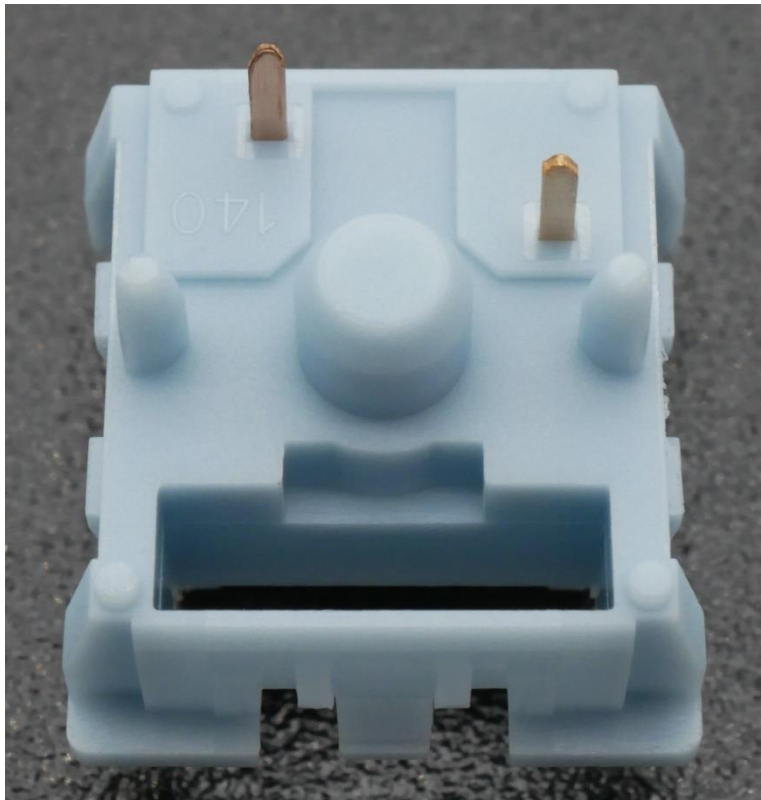
Figure 9: Moyo Studio x XCJZ Snow Grape bottom housing external design showing three-digit mold marking located under the upper metal PCB pin.
