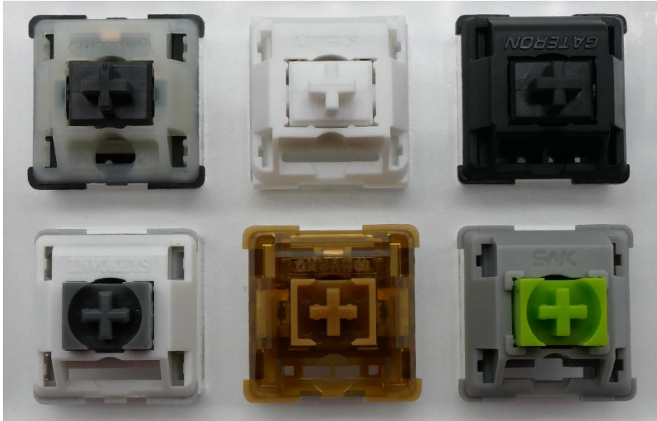
Figure 21: Switches for comparison. (L-R, Top-Bot: Cherry MX 'New Nixie', Novelkeys Dream Cream, Gateron Oil King, Invokeys Black Sesame, Huano Earth Yellow, and Owlabs Neon)
