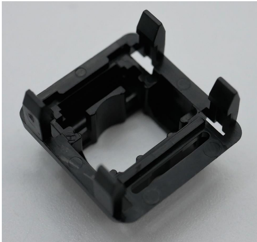
Figure 8: Novelkeys Cream+ top housing internal design featuring mold ejection circles along the upper rim and single, capital letter mold marking in upper left-hand corner of switch stem hole.
