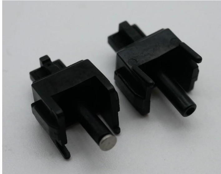
Figure 12: Novelkeys Cream+ stem front and back with titanium insert.
