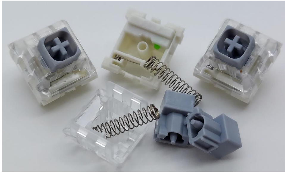
Figure 3: Kailh Box Mute Jade switches and their components.
