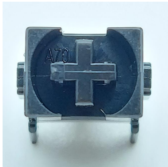
Figure 14: Ultra-high contrast image of Obsidian Pro stem showing both west side injection molding point as well as stem-based mold marking.
