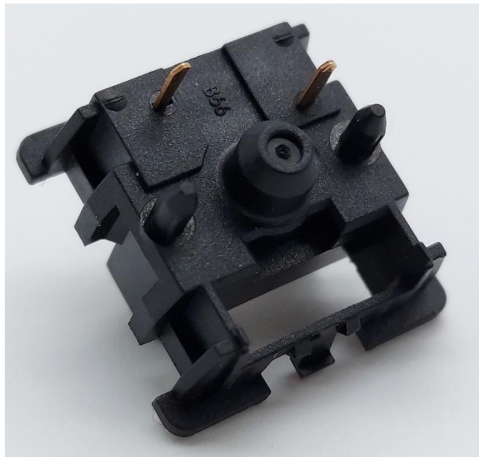
Figure 15: 43Studio's Obsidian Pro bottom housing externals showing polished regions around the PCB mount pins and unique mold marking.
