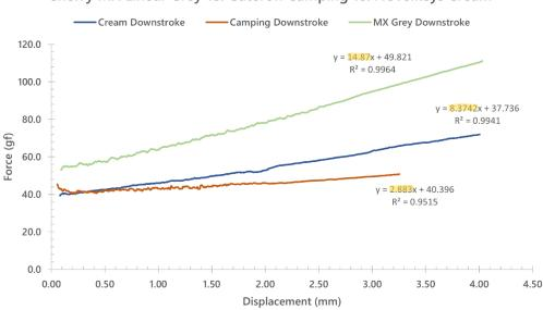
**Figure 1:** Comparison of slopes of the linear region for three different switches with equations for line of best included. Note that the highlighted values correspond to the 'Slope' discussed above.
