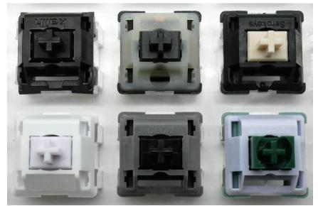
**Figure 8:** Switches for comparison. (L-R, Top-Bot: Novelkeys Cream+ (Titanium Insert), Cherry MX 'New Nixie', Sarokeys BCP, Wuque Studio Morandi, Lubed Black Geon Switch, and Feker Emerald Cabbage)
