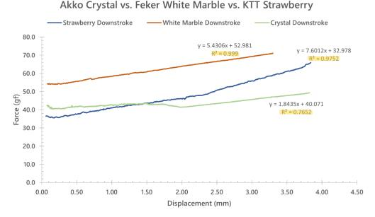
Figure 5: Comparison of flatness of the linear region for three different switches with equations for line of best fit included. Note that the highlighted values correspond to the 'Linearity' discussed above.
