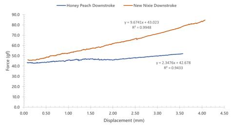
**Figure 3:** Isolated linear region of downstroke force curves for Tecsee Honey Peach and Cherry MX 'New Nixie' switches with equations for line of best fit through each curve.
