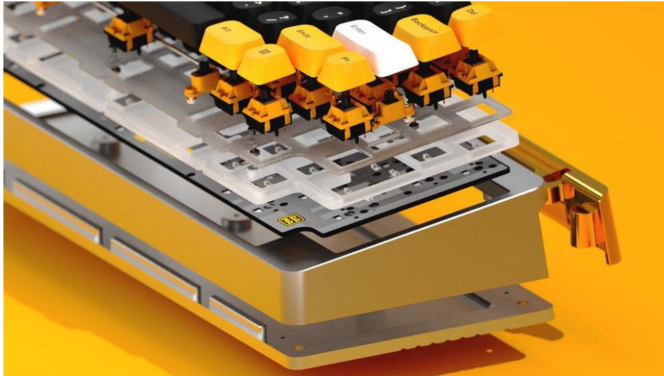
Figure 5: RAMA WORKS M60-A component blowout render showing translucent white MUTE mounting system.
