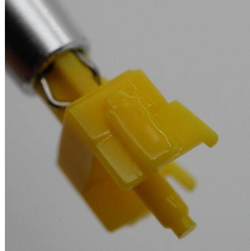
Figure 4: RAMA WORKS Duck stem showing factory lubrication, non-tapered slider rail, and extended central pole.
