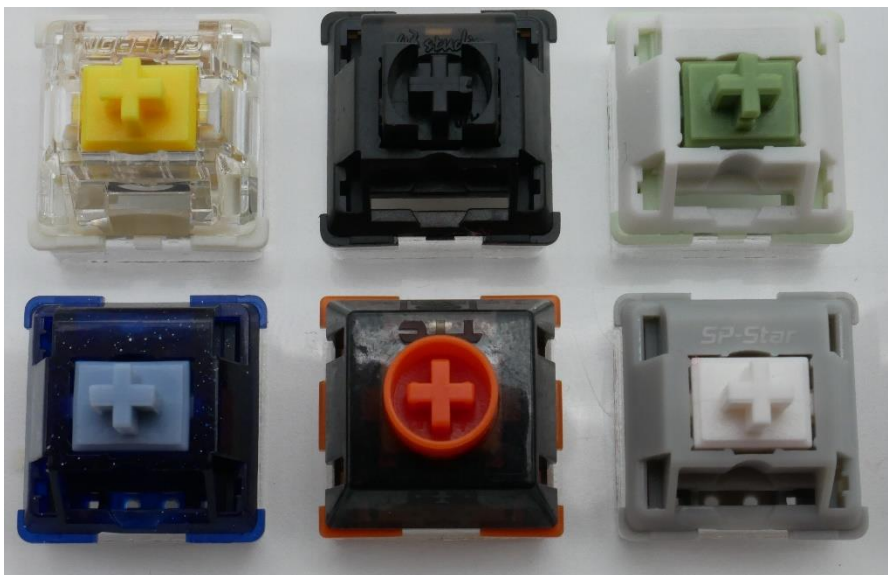
Figure 16: Switches for comparison. (L-R, Top-Bot: Gateron KS9 Pro 2.0 Yellow, Obsidian Pro, Invokeys Matcha Latte, Hoshizora, TTC Tiger, and SP Star Meteor White)
