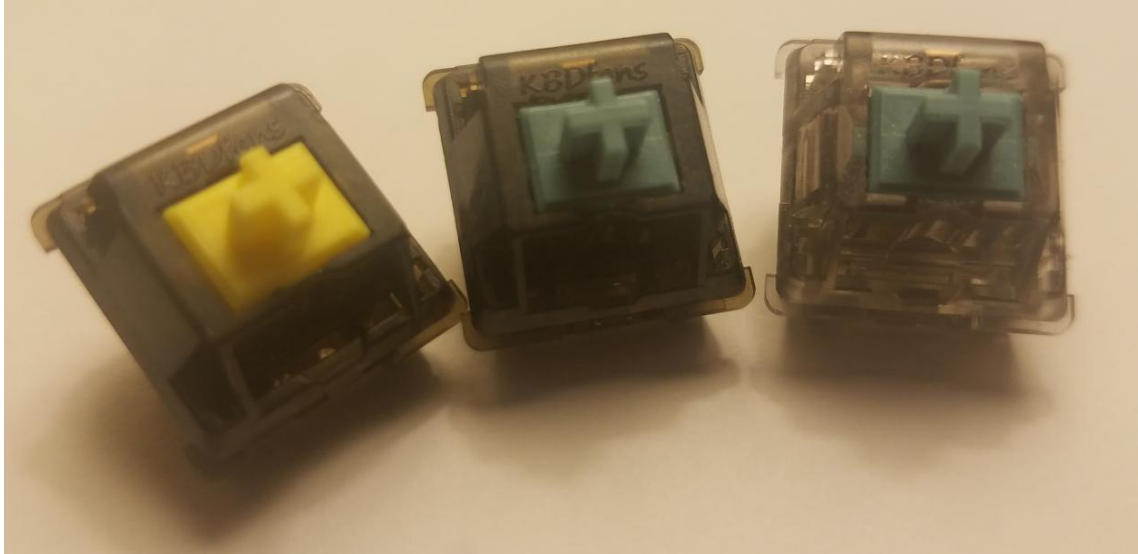
Figure 7: T1 Beta Prototype (Left), T1 Final Prototype (Middle), Stock T1 Night (Right). Note the difference in housing darkness between the prototypes and the release switch. (Personal Collection)
