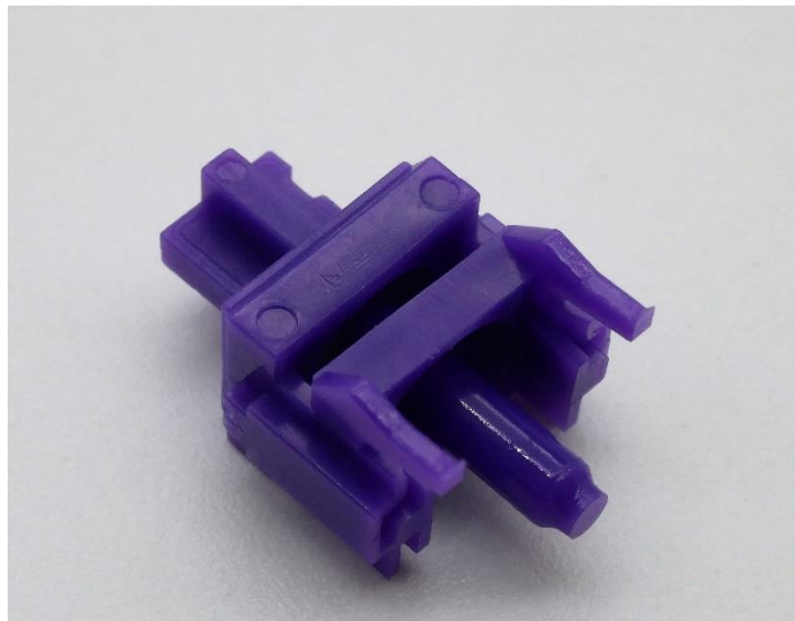
Figure 14: TKC Blackberry stem front plate showing mold ejector circles and movable stem legs of the clicky mechanism.
