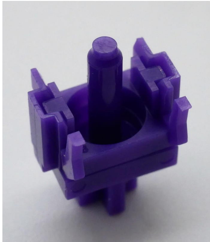
Figure 20: TKC Blackberry stem underside showing how the movable portion is situated within the inner cutout of the affixed portion of the stem with the keycap mount and center pole.
