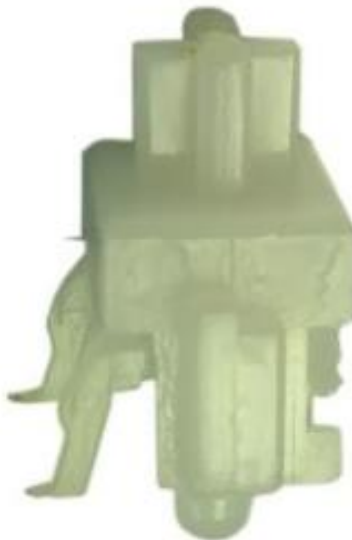
Figure 11: Profile shot of Aristotle White stem from Deskthority showing the original Aristotle click mechanism.
