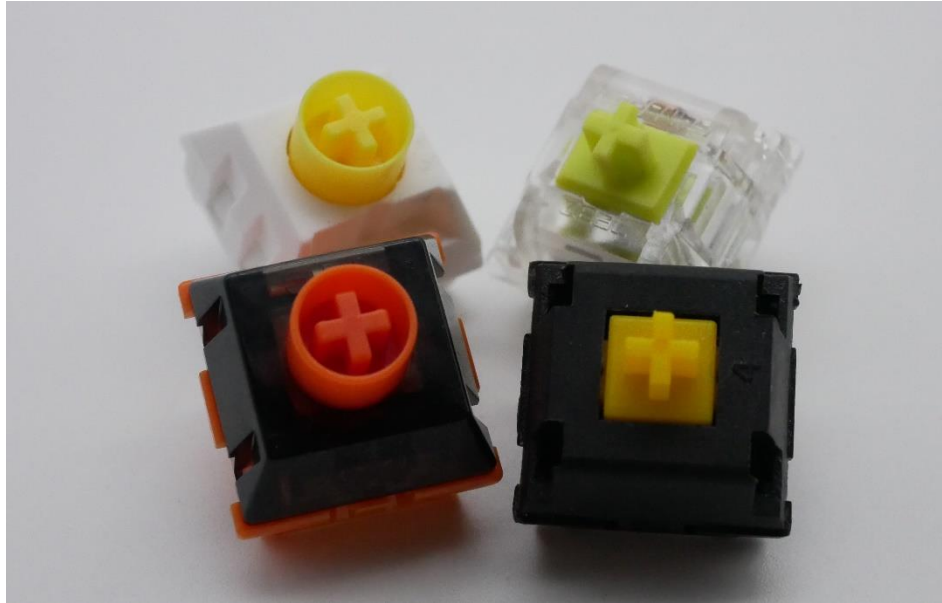
Figure 12: General size comparison between various 'large' MX-footprint switches. (L-R, Top-Bot: Kailh Fried Egg, Zeal Clickiez, TTC Tiger, Taiwan Jet Axis Yellow)
