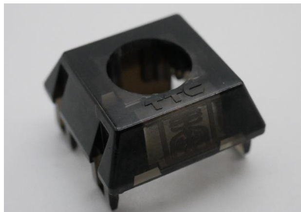
Figure 13: TTC Tiger top housing shot showing TTC nameplate and Ren Yin symbol.
