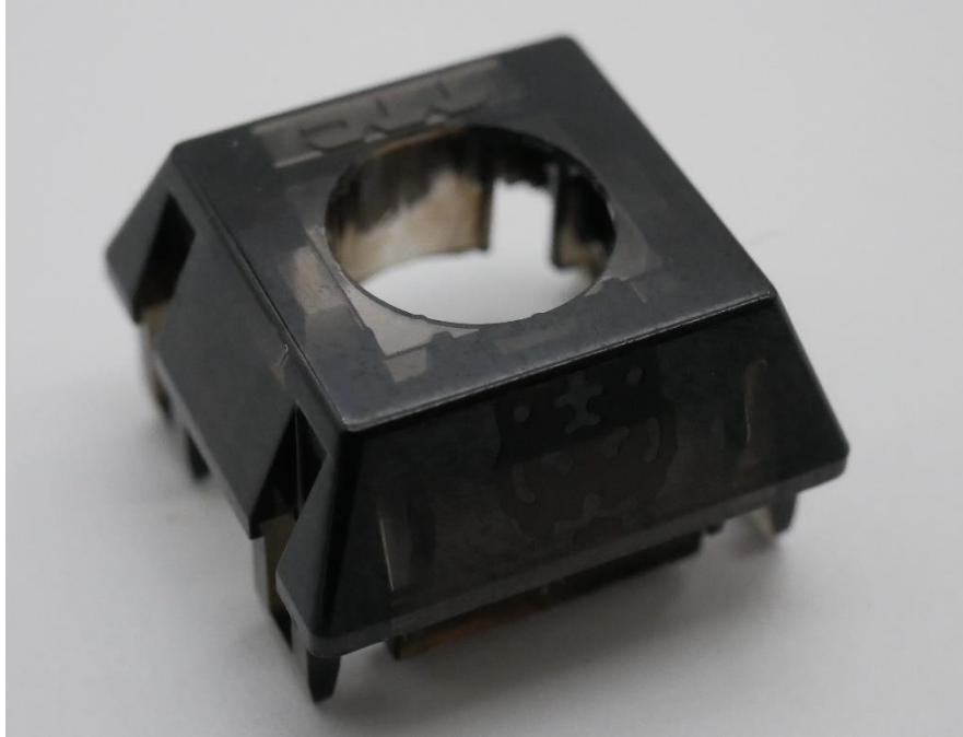
Figure 14: TTC Tiger top housing shot showing grey tiger symbol on the opposite side of the housing from the Ren Yin and TTC logos.
