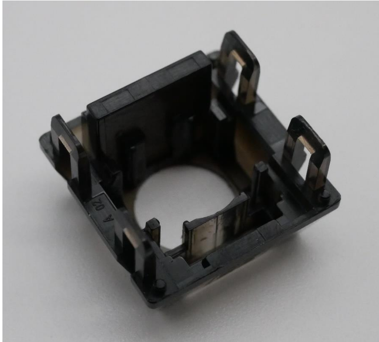
Figure 16: TTC Tiger top housing internal design features showing large LED-blocking outcropping, circular central hole for stem, and hollow attachment pins.
