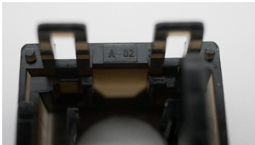
Figure 17: TTC Tiger top housing mold marking closeup.
