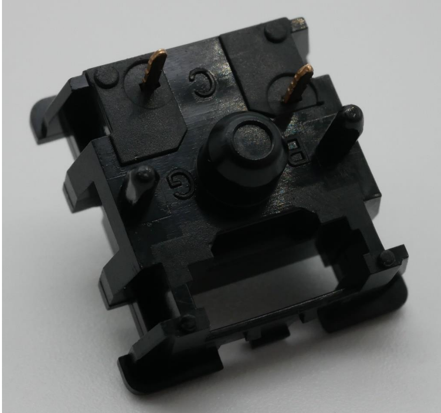
Figure 8: XCJZ Jerrzi Lotus Stem bottom housing exterior design showing PCB mounting pins and locations of three different single letter mold markings.
