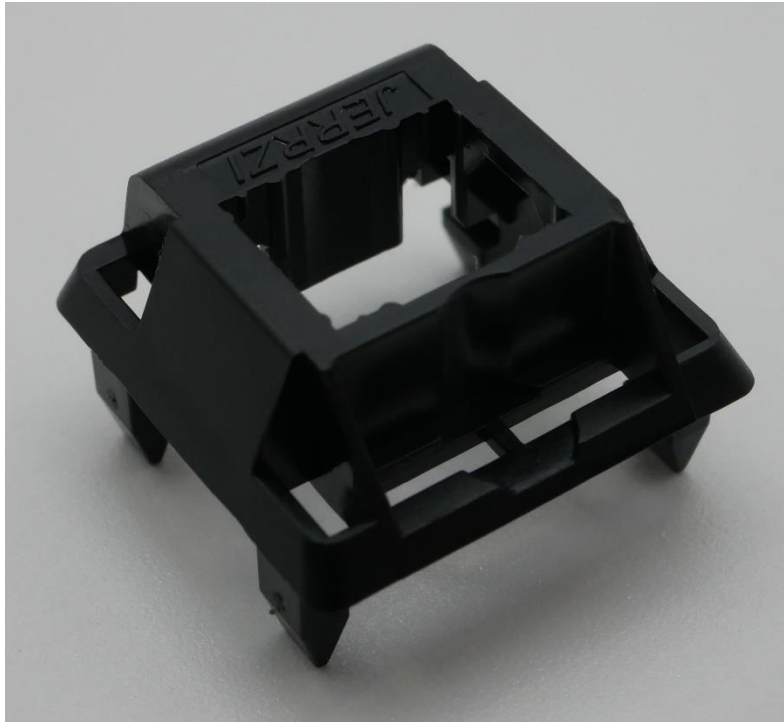
Figure 7: XCJZ Jerrzi Lotus Stem top housing external design showing inverted JERRZI nameplate and bifurcated LED slot with centered circular indentation.
