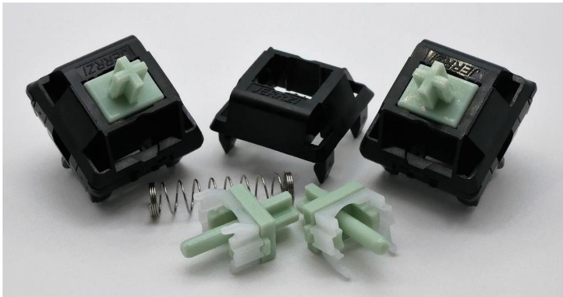
Figure 6: XCJZ Jerrzi Lotus Stem switch and its components.
