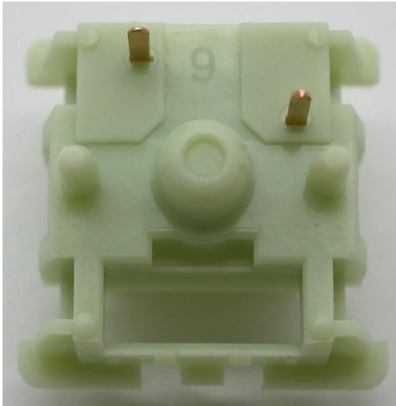
Figure 10: Zaku II bottom housing exterior design showing 5-pin/PCB mount construction and inverted, single number mold marking in location similar to that of other Tecsee switch releases over the years.
