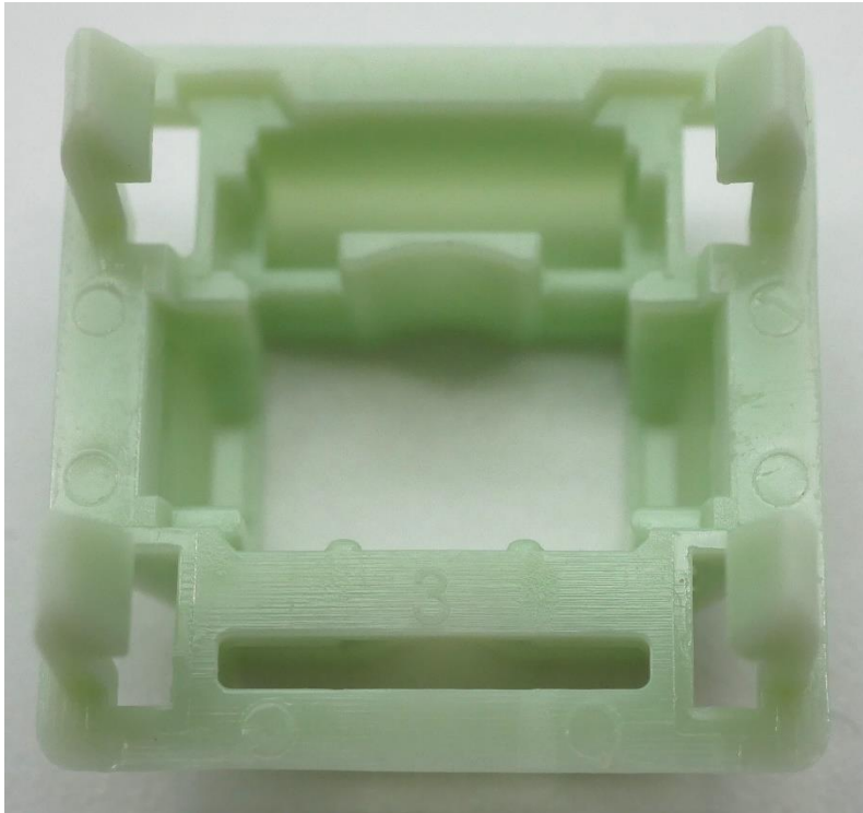
Figure 7: Zaku II top housing internal design showing mold ejector circles on all edges of switch as well as single number mold marking on the interior edge of the LED/diode slot as commonly seen in Tecsee switches.
