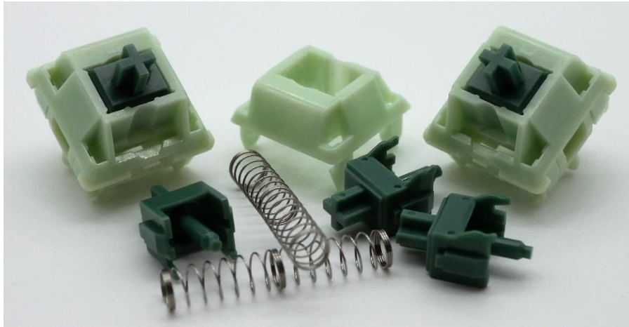
Figure 3: Zaku II switches and their components.
