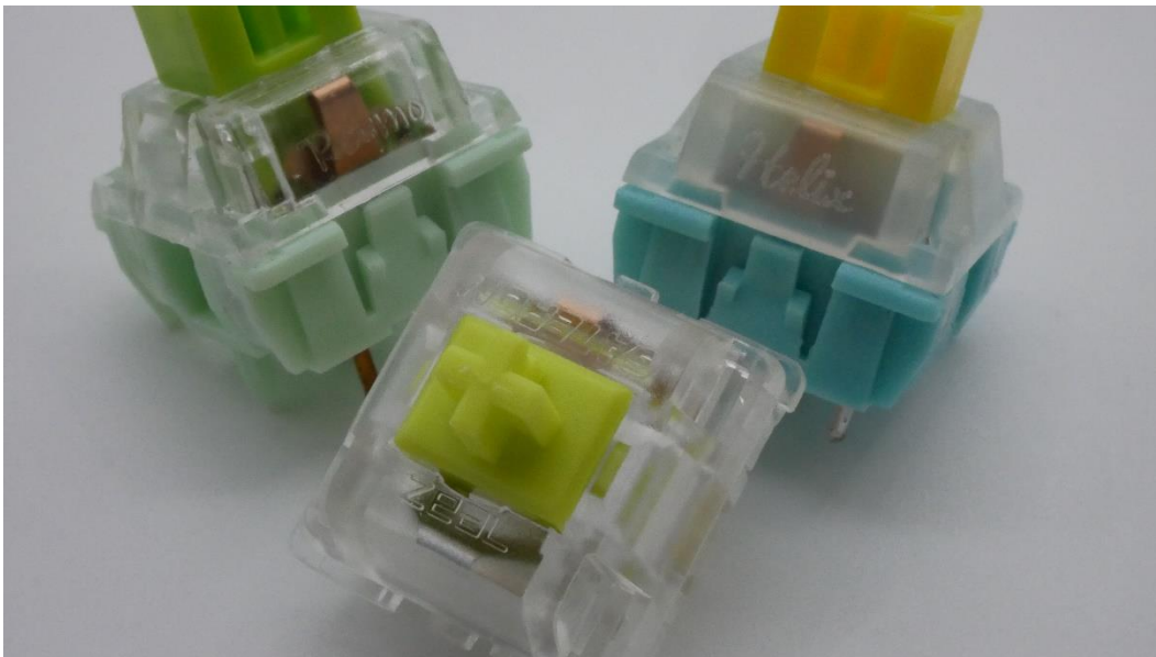
Figure 9: Family photo of modern, MX style switches featuring multiple top housing engravings including TTC Ace (Top Left), TTC x Helix Lab Skylar (Top Right), and Zeal Clickiez 75g. (Front Center).
