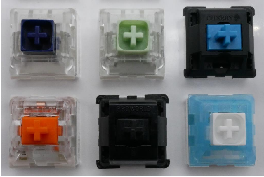
Figure 21: Switches for comparison in the clicky mode. (L-R, Top-Bot: Kailh Box Navy, Kailh Box Jade, Cherry MX Blue, Novelkeys Sherbet, ProWorld Clicky, and Kailh Arctic Fox)
