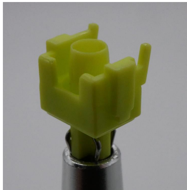
Figure 9: Clickiez 75g. stem showing squared off backplate, non-tapered slider rails, and CAP like central pole design.
