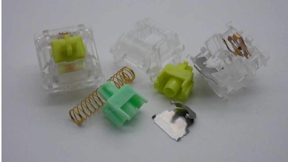
Figure 8: Zeal Clickiez switches and their components.
