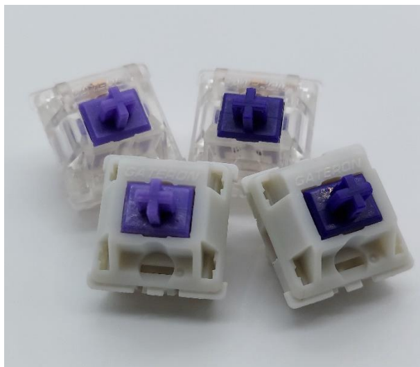
Figure 8: Stem color comparisons between Zealios V1 62g and 67g (back) and Zealios V1 Redux 62g and 67g switches (front).
