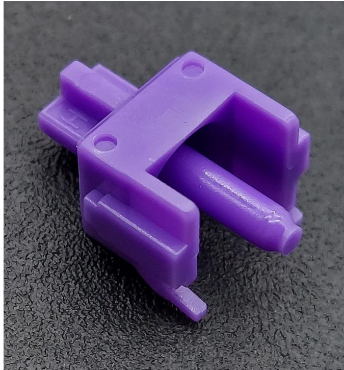
Figure 12: Zealio V1 Redux 62g stem backside shot showing distinctive features such as non-tapered slider rails, high set mold ejector marks on backplate, and slightly tapered center pole.
