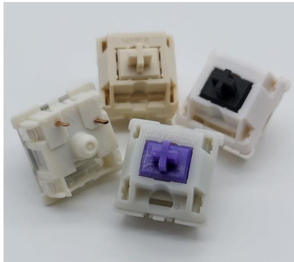
Figure 9: White and white-adjacent colored switch comparisons to Zealio V1 Redux (front). (L-R: Gateron Black, Novelkeys Cream, Moyu Black)
