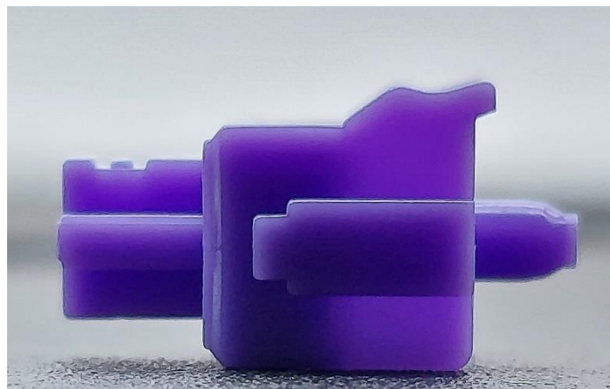
Figure 11: Side profile shot of Zealio V1 Redux 62g stem showing tactile bump profile.
