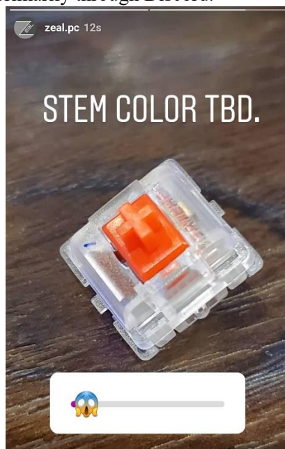
Figure 4: 1st Zeal 3-in-1 switch prototype photo featuring orange stem.
